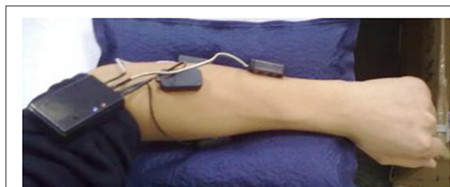
FIGURE 4 | Multichannel wireless surface EMG acquisition device.
