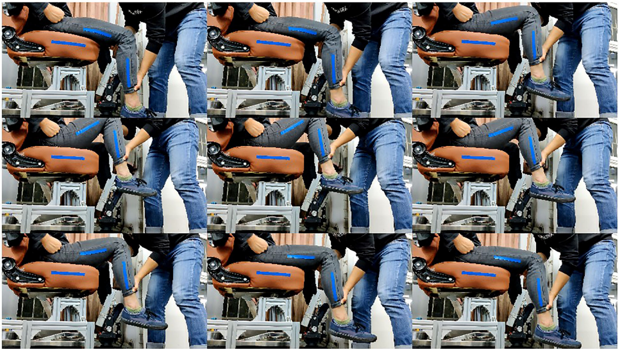
FIGURE 5 | Measurement of the hip joint range of motion in the sagittal plane.
