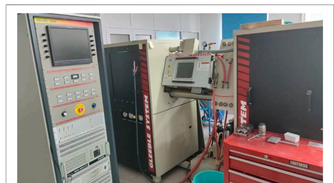
FIGURE 3 | Gleeble-3800 compression test setup.
