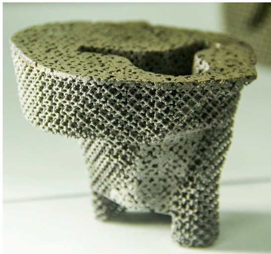
FIGURE 4 Personalized porous tantalum prosthesis printed by pure tantalum.
