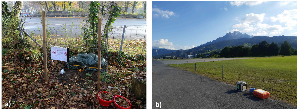
FIGURE 4 | (A) LUZ02—example of the station of the temporary network. (B) Example of measurement of ambient noise during the survey in June 2020. The setup consists of a Lennartz 5-s sensor and Centaur digitizer.
