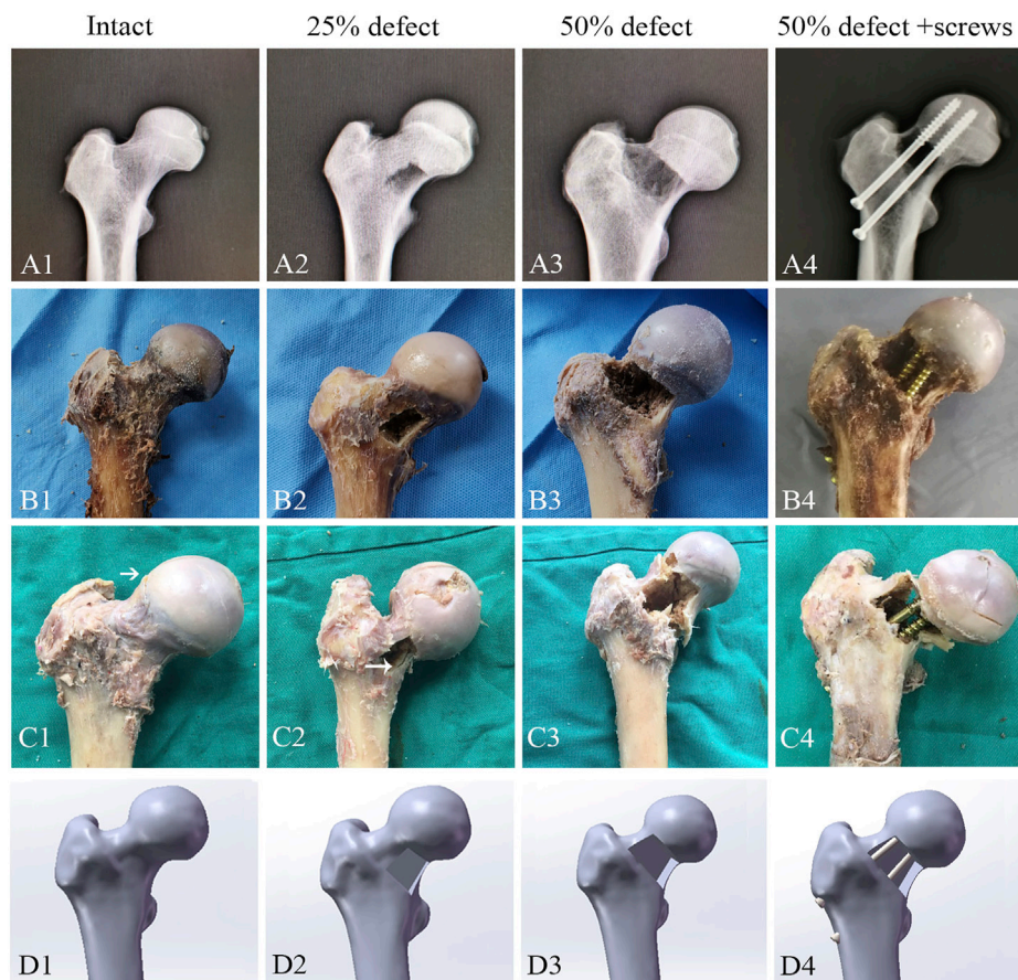
FIGURE 2 | Representative images for X-ray ( A1–A4 ), cadaveric tests ( B1–B4 ), femoral neck fracture ( C1–C4 ), and FEA ( D1–D4 ) of the control group, 25%-defect group, 50%-defect group, and 50%-defect + two cannulated screw group.
