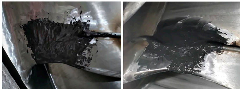
FIGURE 6 | The photos of protection of the strain gauges by metal protective coating.
