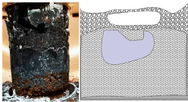
FIGURE 2 | Morphology of the corium ingot after the experiment (2).
