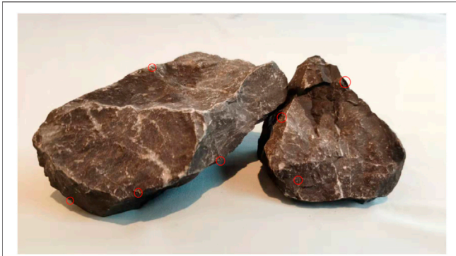
FIGURE 4 | There are many small indentations on the surface of the aquarium stones (small red circles). In their MRI image, those indentations that meet the CAF standard are used as characteristic areas, to improve the measurement accuracy.
