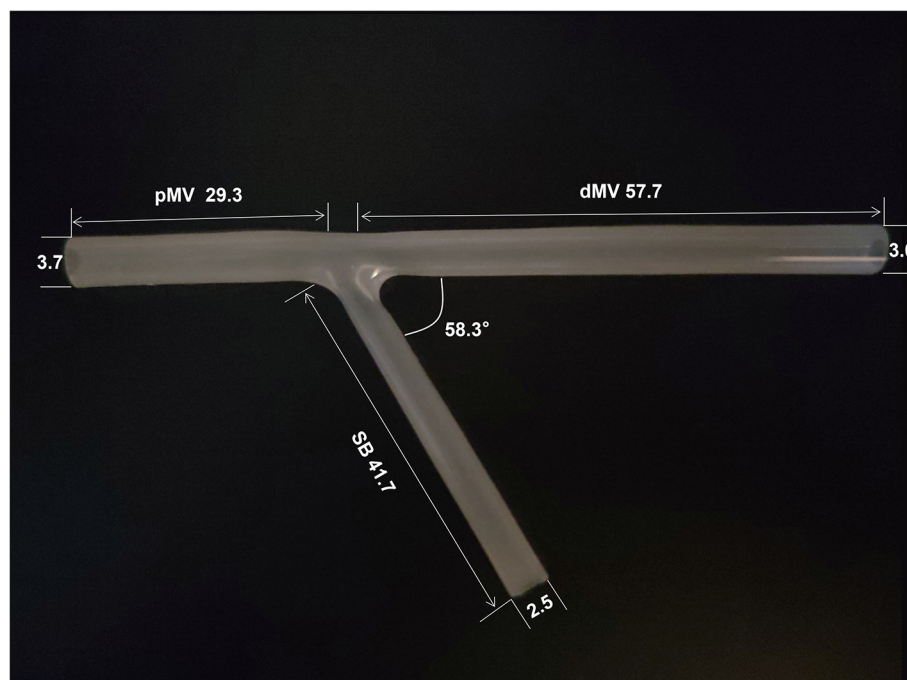
FIGURE 2 | Bench test model of bifurcation stenting. The length of the pMV, dMV and SB is 29.3, 57.7 and 41.7 mm respectively. The inner lumen diameter of the pMV, dMV and SB is 3.7, 3.0 and 2.5 mm respectively. The bifurcation angle is 58.3°. pMV, proximal main vessel; dMV, distal main vessel; SB, side branch.
