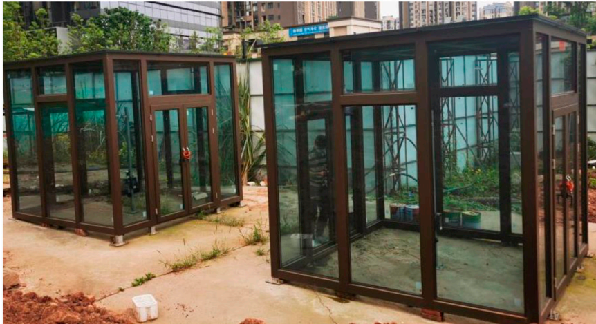
FIGURE 6 | Comparison of thermochromic glass and ordinary Low-E glass sunlight room.
