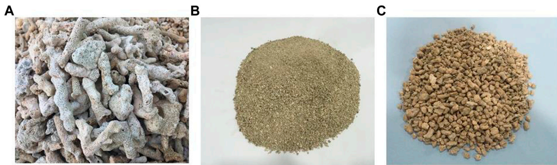
FIGURE 2 | (A) Corals; (B) coral fine aggregate; (C) coral coarse aggregate (Huang et al., 2020a).
