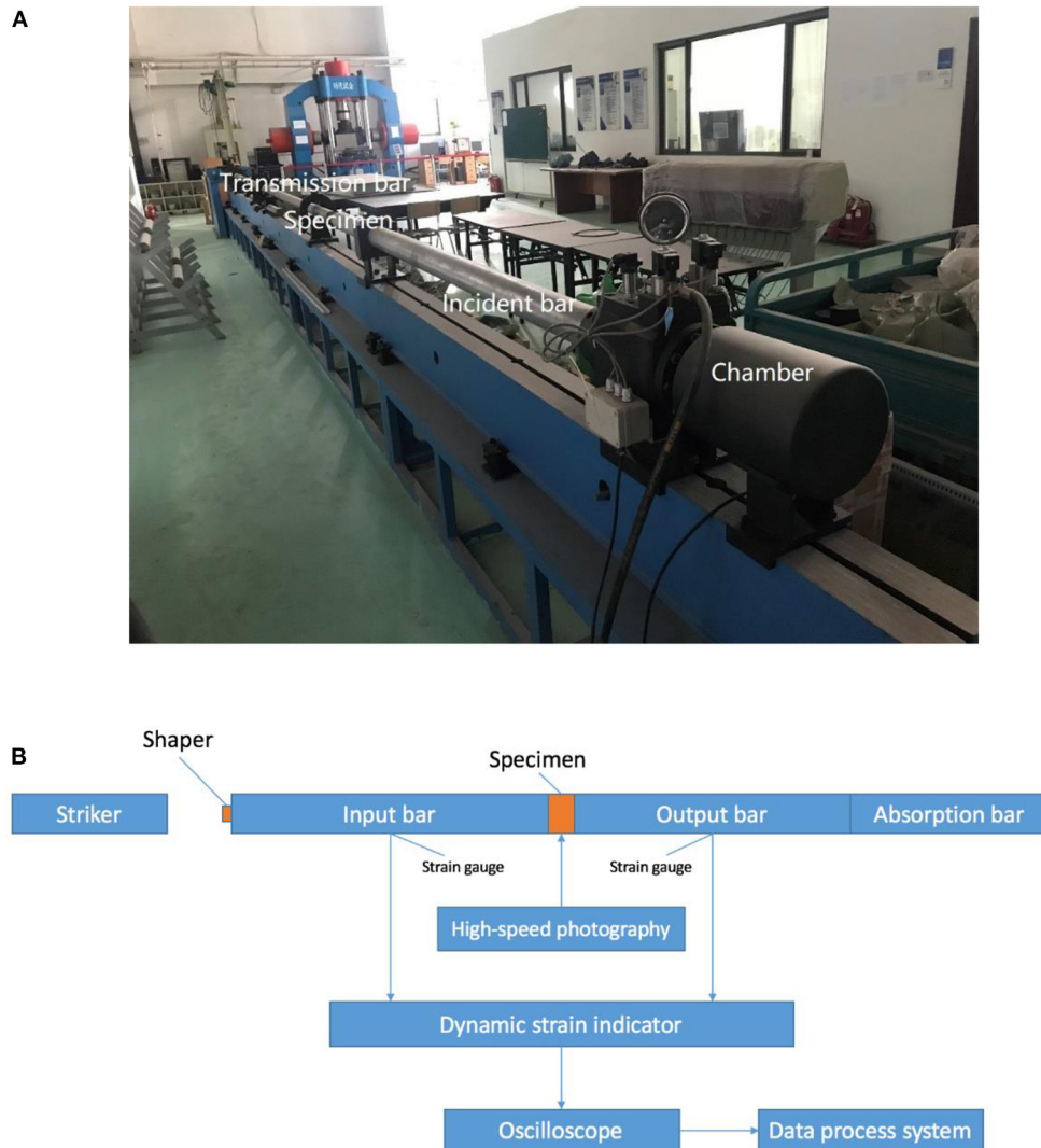
FIGURE 2 | SHPB test system (A) photograph (B) schematic illustration.
