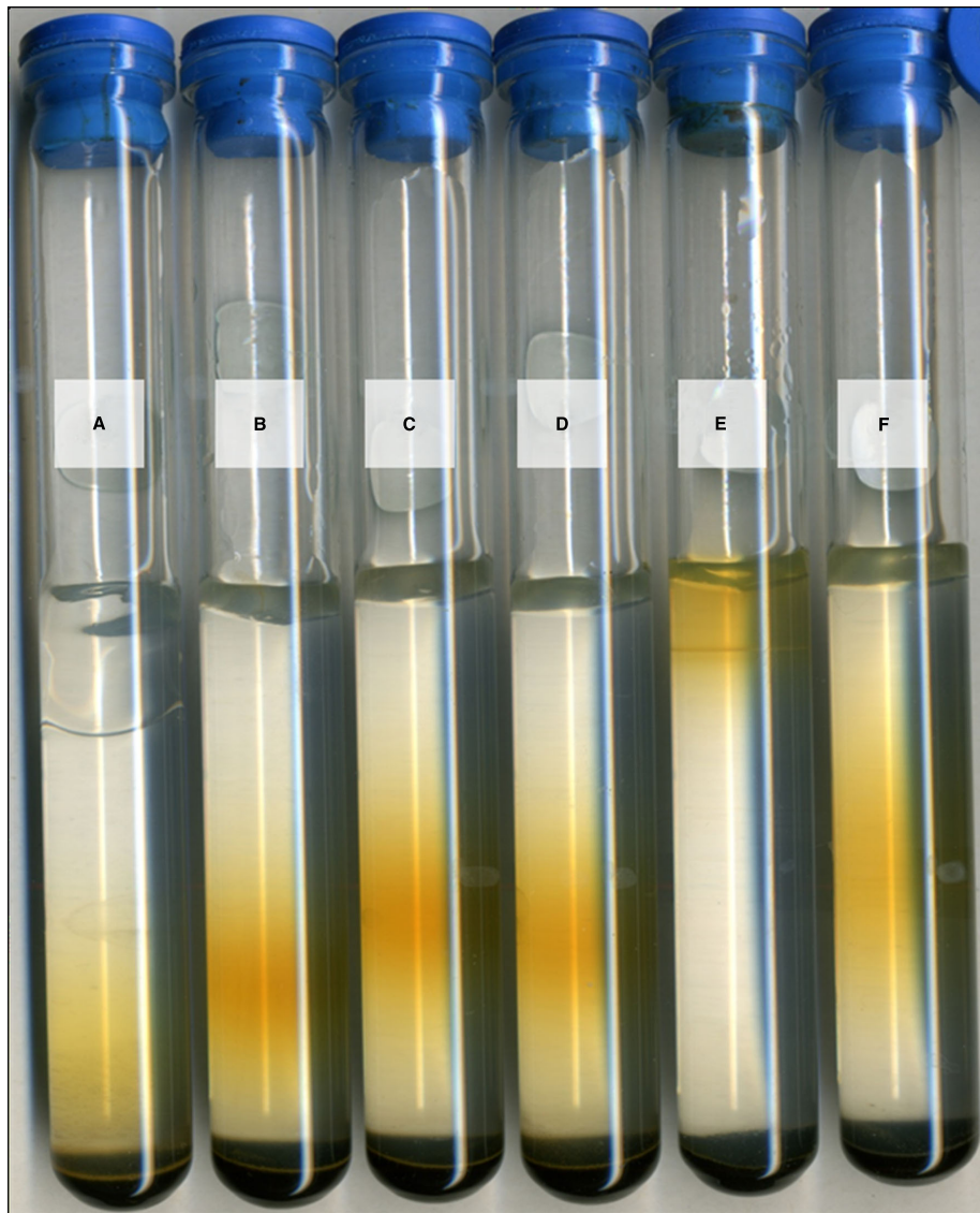
FIGURE 5 | Fe(II) oxidation under respiratory inhibition.
