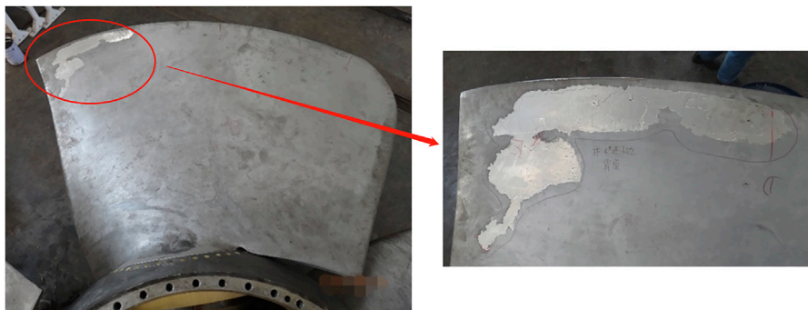
FIGURE 5 | Blade cavitation of tubular turbine (Shengyang, 2020).
