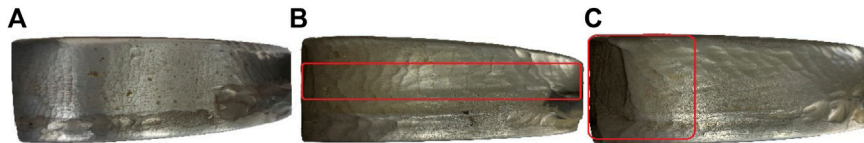
FIGURE 7 | Pressure surface wear under different mass concentration. (A) 15%, (B) 20%, and (C) 30%.
