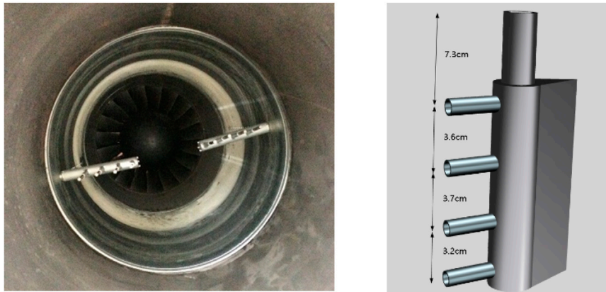
FIGURE 12 | Photo and 3D design drawing of radial rakes.
