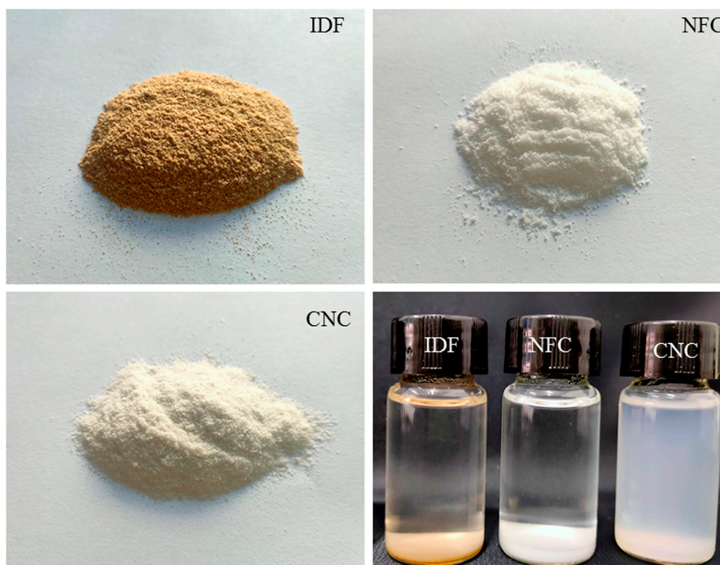
FIGURE 1 | Photographs of IDF, NFC, and CNC powders and their aqueous suspensions after setting aside at room temperature for 24 h.
