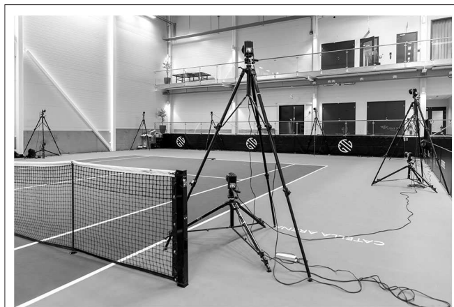
FIGURE 1 | Picture of the calibrated measuring volume with the majority of the motion capture cameras visible.
