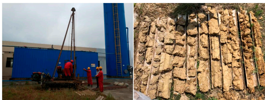
FIGURE 4 Drilling site and soil core sampling process.
