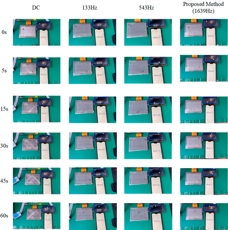
FIGURE 12 Asymmetric AC driving results at different frequencies.
