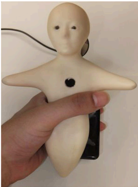
FIGURE 1 | Elfoïd: cellular phone-type teleoperated android.
