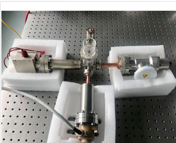
FIGURE 11 The miniaturized vacuum system.
