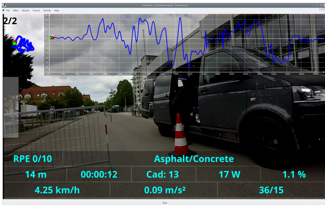
FIGURE 4 | Screenshot from a Powerbike simulation of a ride on a real-world track. The playback speed of a video recorded on the track is controlled by the pedaling speed and the ergometer brake force simulates the incline of the track. The software enables the acquisition of various cycling performance parameters like cadence, pedaling power, cycling speed, acceleration, and distribution of the power over the pedaling cycle. The blue curves in the top represent the map and the slope profile of the simulated track. The Powerbike simulation software could serve as a virtual reality environment for the BrainCycles setup, enabling studies with visual feedback or simulating real-world bicycle navigation in patients with movement disorders.
