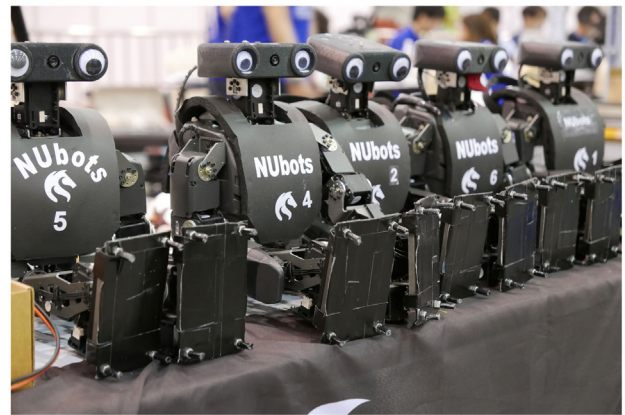
FIGURE 11 | Modified Darwin-OPs of the 2015 NUbots team equipped with new 3D-printed heads using a higher resolution camera, padded jackets to soften falls, and soccer studs to improve grip on artificial grass.
