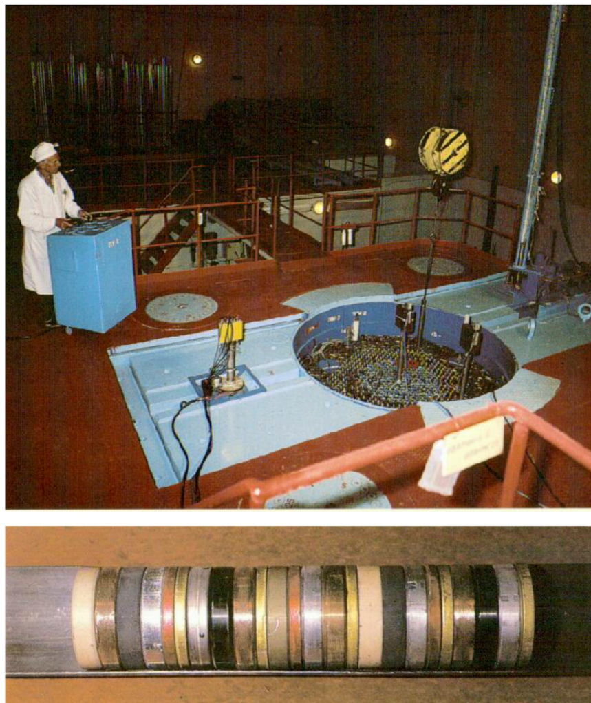
FIGURE 2 BFS-1 critical facility (Top) and example fuel pellet loading (Bottom).
