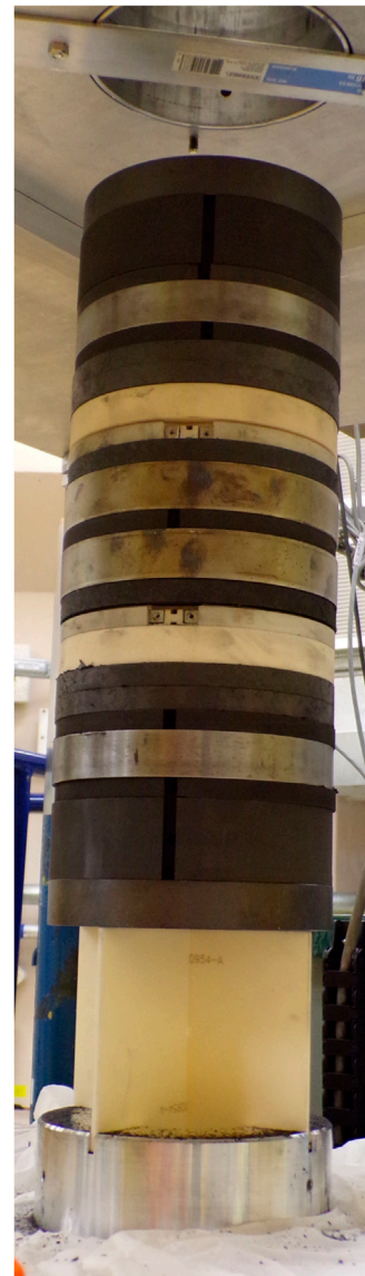
FIGURE 8 Photo of the core stack during the Hypatia experiment.
