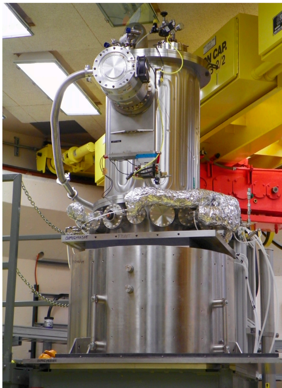
FIGURE 10 Photo of the KRUSTY experiment on the Comet assembly.
