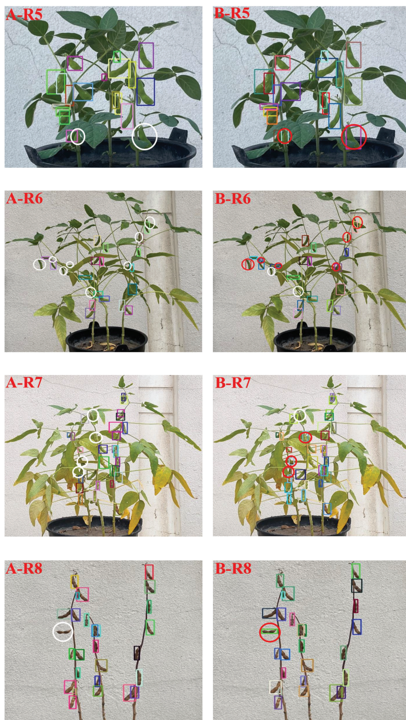
FIGURE 12 Comparison of partial recognition results before and after model improvement (A) YOLOv5 model; (B) Improved YOLOv5 model.
