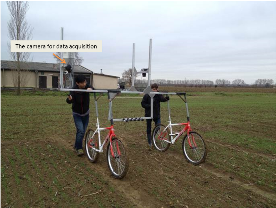
FIGURE 1 | The image acquisition in the field with the Phenotypette.
