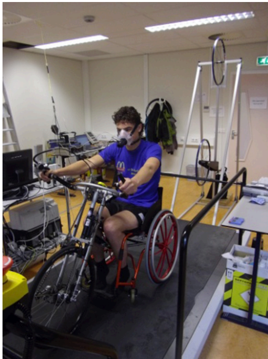
FIGURE 1 | The experimental handcycle, consisting of a wheelchair with a mounted handcycling unit in front of the pulley system on the motor driven treadmill.
