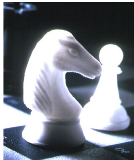
FIGURE 1 | Apatite–mullite chess piece cast to shape by the lost wax method.
