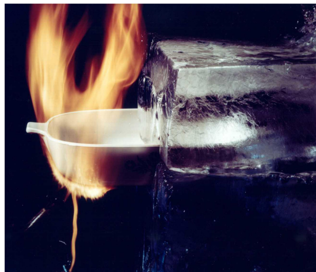
FIGURE 8 | Thermal shock resistance of Corningware® demonstrated.
