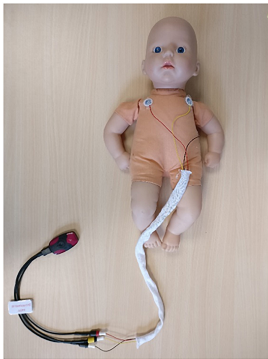
FIGURE 1 | Portable ECG recorder and thoracic setup. Three ECG electrodes were fed through an alignment sleeve to reduce the distance between ECG wires and prevent magnetic induction artifacts on raw ECG signal (500 Hz with automatic R-peak detection).
