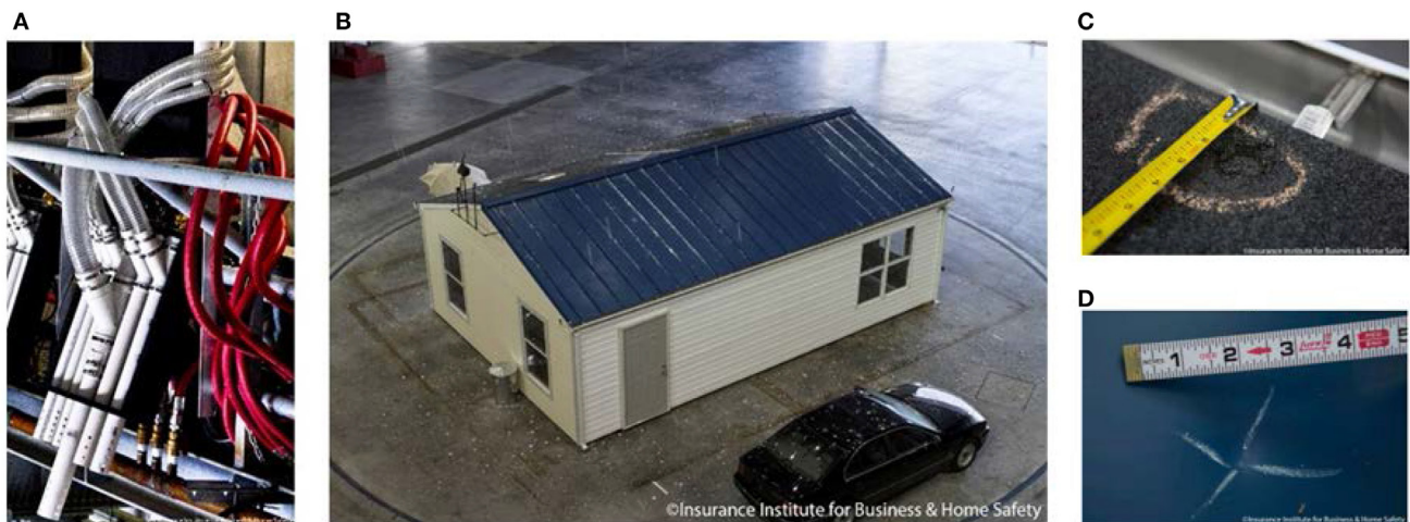
FIGURE 13 | (A) One of 12 cannons, featuring 6 impact barrels, located in the test chamber at the IBHS Research Center. (B) IBHS full-scale hailstorm demonstration in 2013. (C) Damage on a 3-tab shingle on the test specimen. (D) Damage on the metal roof on the test specimen.
