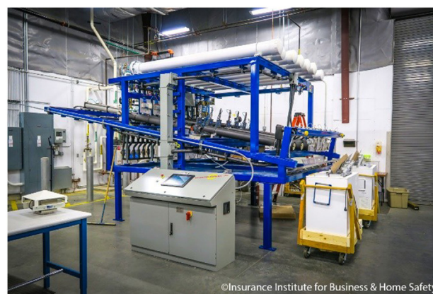
FIGURE 11 | IBHS Hail Machine that was developed with Accudyne Systems Inc., to mass produce laboratory hailstones, which mimic material properties of natural hail.
