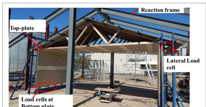
FIGURE 9 | Full-scale tests on house cross-section.
