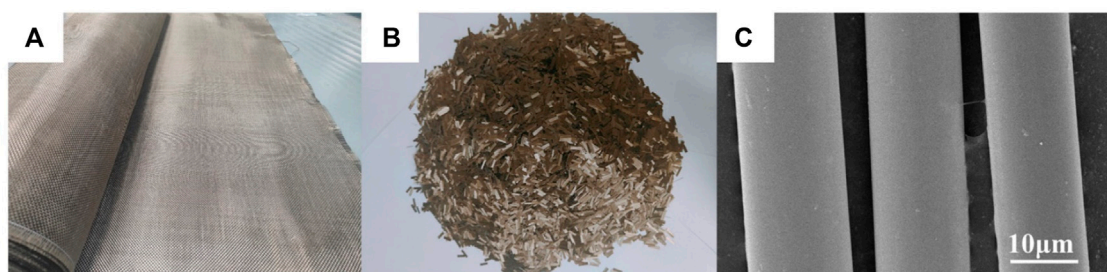
FIGURE 12 Basalt fiber's physical appearance, (A) sheet, (B) short fibers, and (C) SEM image of basalt fiber (Liu H. et al., 2022).
