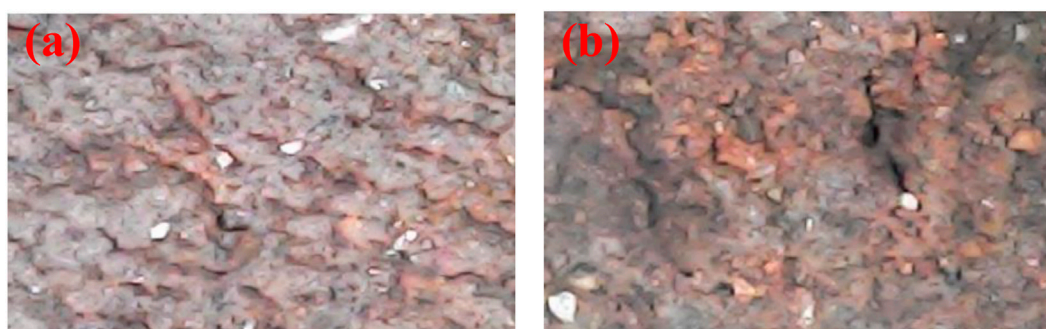
FIGURE 7 Pile tip mudstone images of normal and damaged piles in static load tests. (A) Normal pile. (B) Pile with static load failure. 1, collet; 2, press; 3, penetration scale; 4, penetration force scale; 5, indicator ring; 6, rear cover; 7, diagram of the needle penetration ratio and uniaxial compressive strength; 8, penetration needle.
