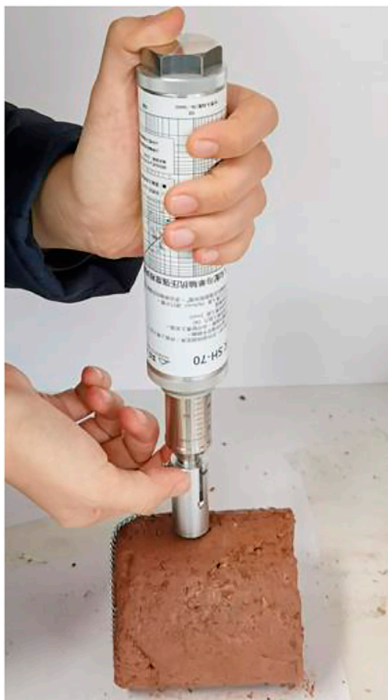
FIGURE 9 Needle penetration test on a mudstone core.
