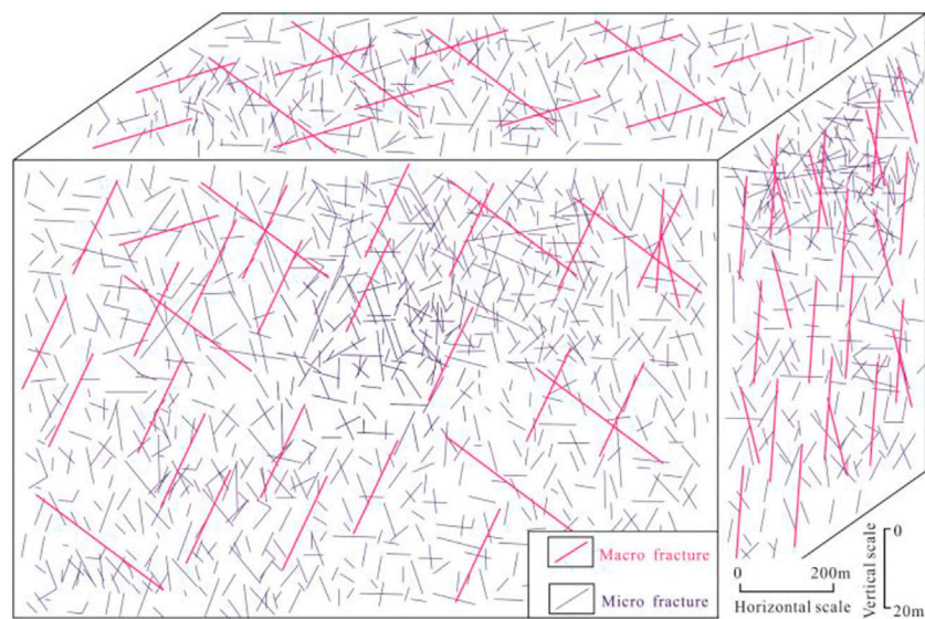
FIGURE 13 Schematic diagram of small-scale fracture network with high-density and multi-sets.
