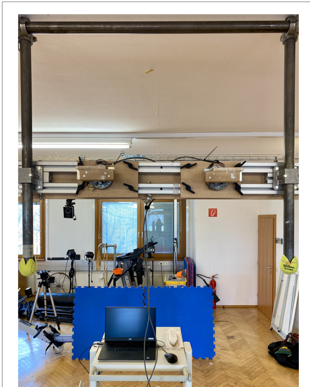
FIGURE 1 Instrumented hang board used in the study. The force sensors were placed in separate hand holds, with height and width being adjusted according to participant's individual anthropometry and the desired arm lock-off angles required in the tasks.
