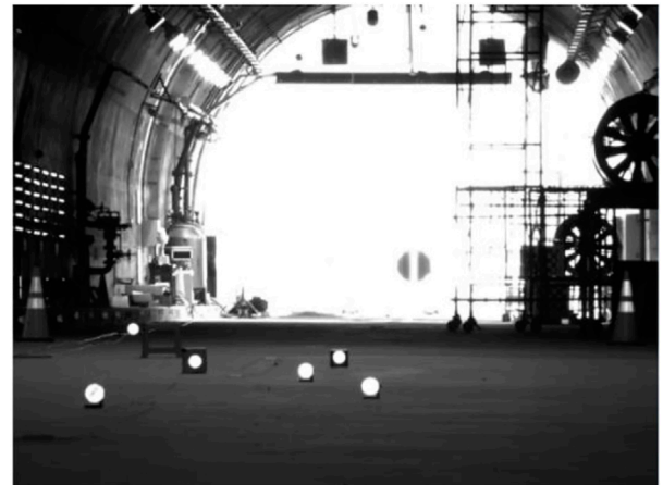
FIGURE 2 Imaging effect of circular reflective mark.
