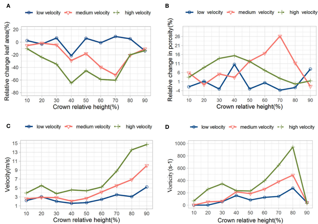
FIGURE 11 Changes in windward area (A), porosity (B), velocity (C), and vorticity (D) at different CRHs.
