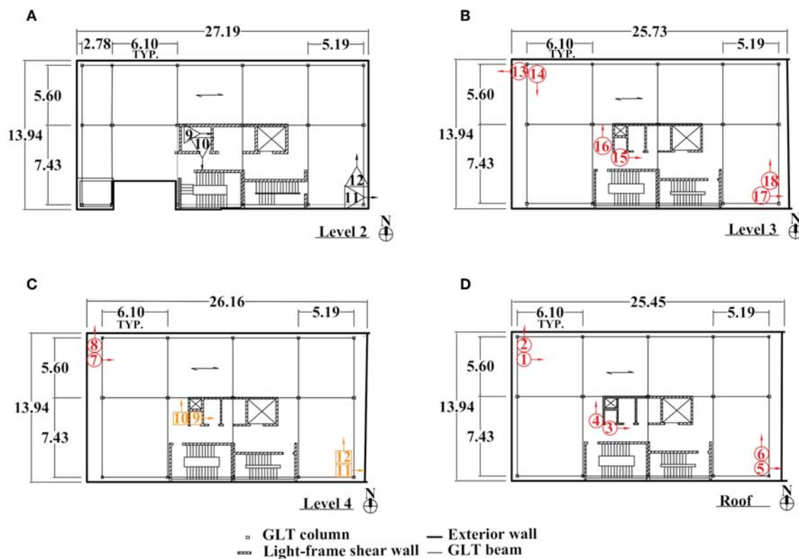
FIGURE 2 | Floor level plans showing the locations of accelerometers marked 1–18. Accelerometers 1–8 and 13–18, shown in red circles are the reference accelerometers. Roving accelerometers 9–12 are shown in yellow squares for setup 1 and black triangles for setup 2. The dimensions are presented in meters. (A) Second floor level, (B) Third floor level, (C) Fourth floor level, (D) Roof level.
