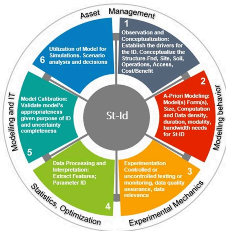
FIGURE 4 | Steps of structural systems identification.
