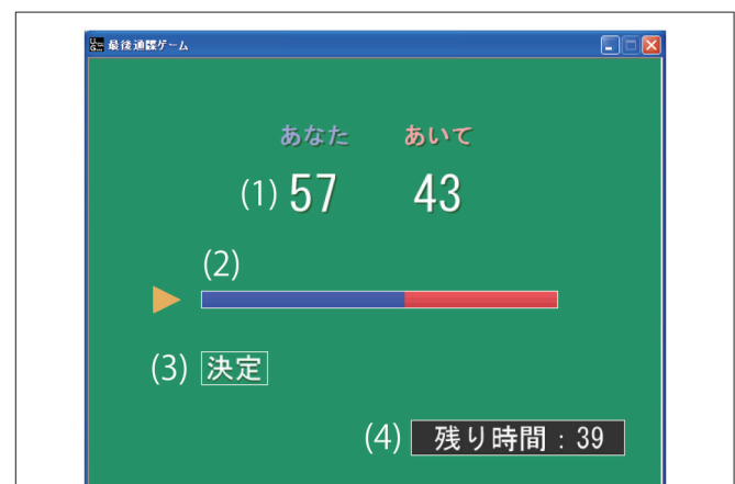
FIGURE 1 | Graphical user interface used by the proposer to determine the offer: (1) numerical representation of the offer, (2) slider bar to change the offer, (3) button for final decision, and (4) time remaining.
