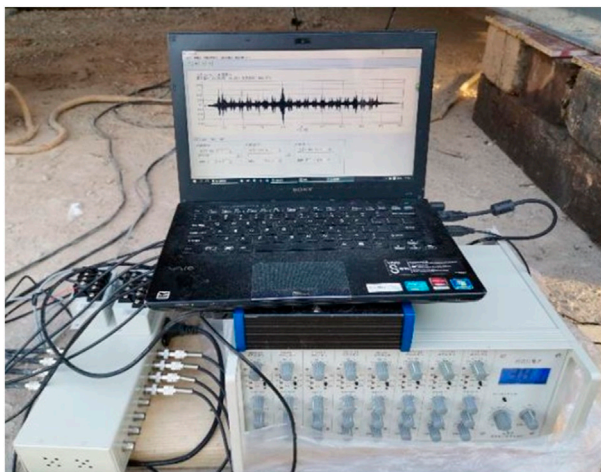
FIGURE 4 Field-measured data diagram of a passing train.
