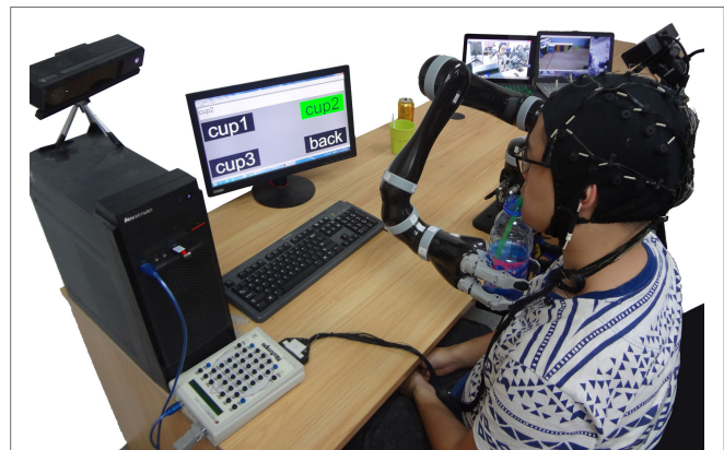
FIGURE 13 | The ID-SIR system assists a user for drinking (the individual agrees to publish his photo).
