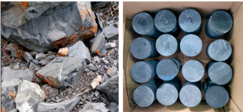
FIGURE 2 Complete rock and prepared standard rock specimens.
