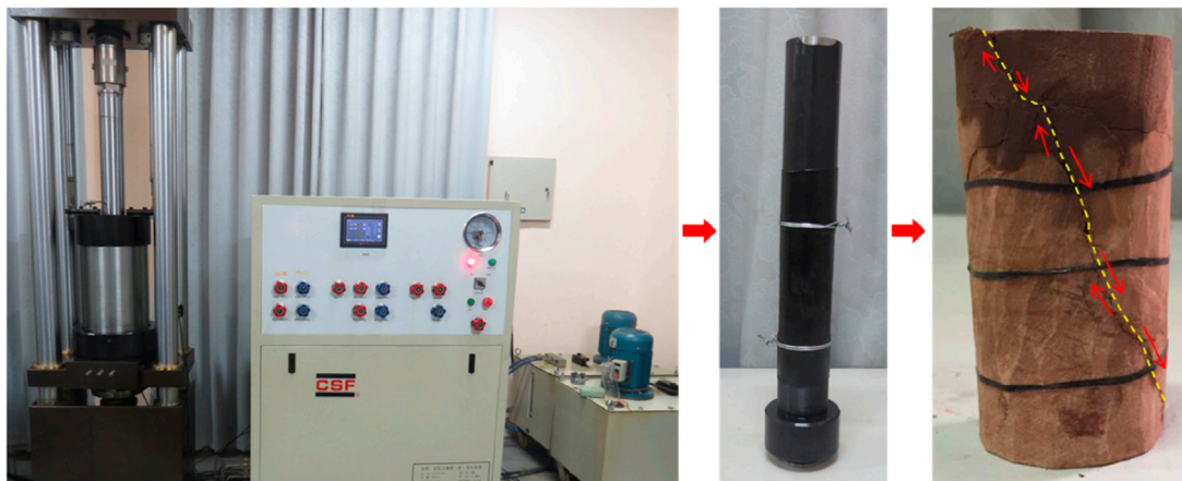
FIGURE 2 Experimental setup of the long-term creep test.
