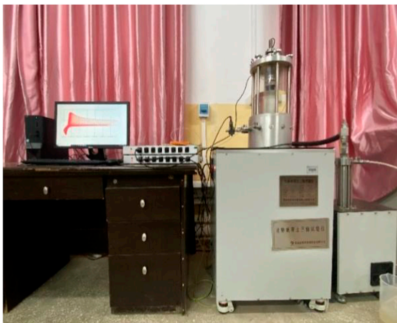
FIGURE 2 KTL-DYN10 dynamic triaxial equipment.
