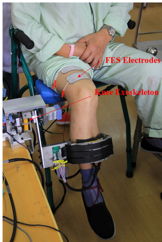
FIGURE 3 | Experimental setup of hybrid FES-exoskeleton rehabilitation system (FEXO Knee). A paralyzed patient (P3) wearing FEXO Knee was taking experiment, where outer shell of exoskeleton held the shank, and FES electrodes were attached to skin over targeted muscles (quadriceps and hamstrings).
