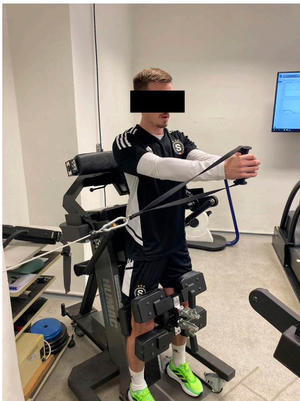
FIGURE 1 Maximal voluntary contraction test of trunk rotational strength using the isometric mode of the Humac NORM dynamometer with trunk modular and wheel components (CSMi, Stoughton, MA, United States).
