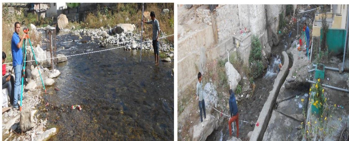
FIGURE 3 Cross-sectional plotting and discharge measurement using the current meter.
