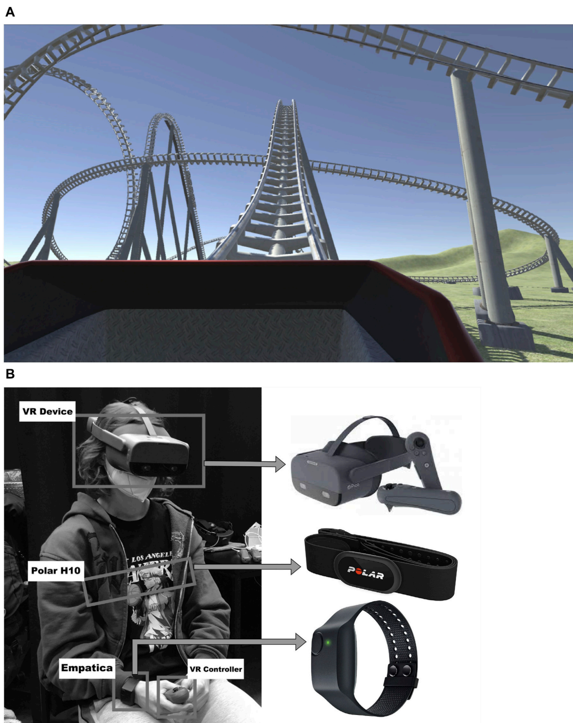
FIGURE 1 The overview of the CS detection setup. (A) Screenshot of the virtual roller coaster environment used to intentionally induce CS. (B) An equipped participant (center) and the respective sensors used during the experiments in detail.
