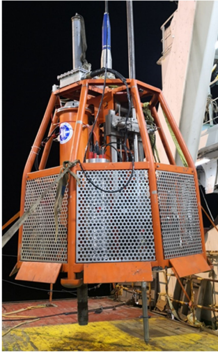
FIGURE 2 Seabed penetration platform: (A) Mechanical structure diagram; (B) picture of equipment used for field application.
