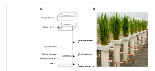
Schematic diagram of experimental device for collecting underground leaching water from farmland [(A) is design drawing and (B) is
