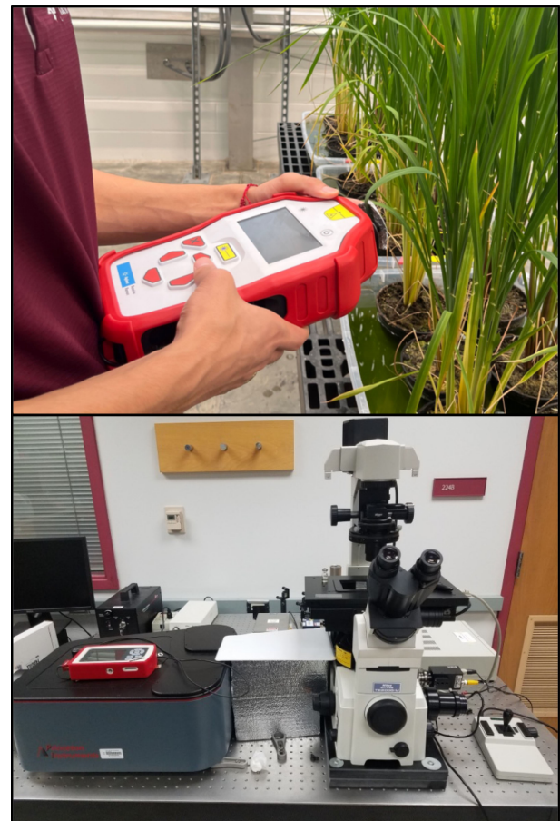
FIGURE 1 Commercially available hand-held Raman spectrometer with 830 nm excitations (top) and a bench-top home-built confocal Raman microscope (bottom).
