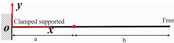
FIGURE 2 Cantilever beam model with a single concentrated mass point.
