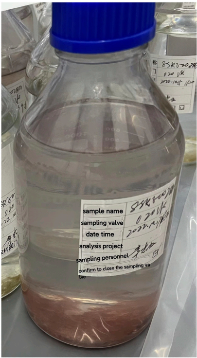
FIGURE 9 Flocculent precipitation at the bottom of the SRE system sample.
