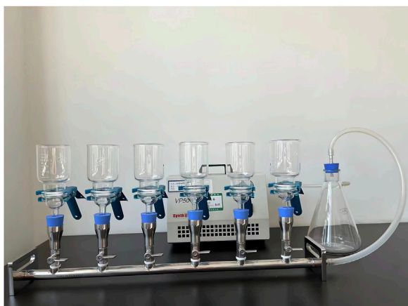
FIGURE 2 Photo of the filter extraction unit.
