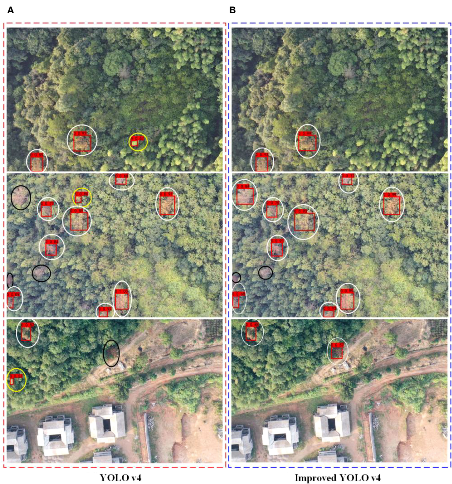
FIGURE 12 Remote sensing image recognition results under strong light environment. * white circles indicate correct detections, black circles indicate missed detections, yellow circles indicate misdetections. (A) YOLO v4 detection results (B) Improved YOLO v4 detection results.
